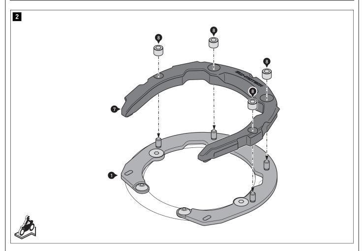
Carefully screw the tank ring [7] to the mounting ring [1].
