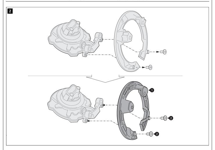
Unscrew the screws from the cap unit.
