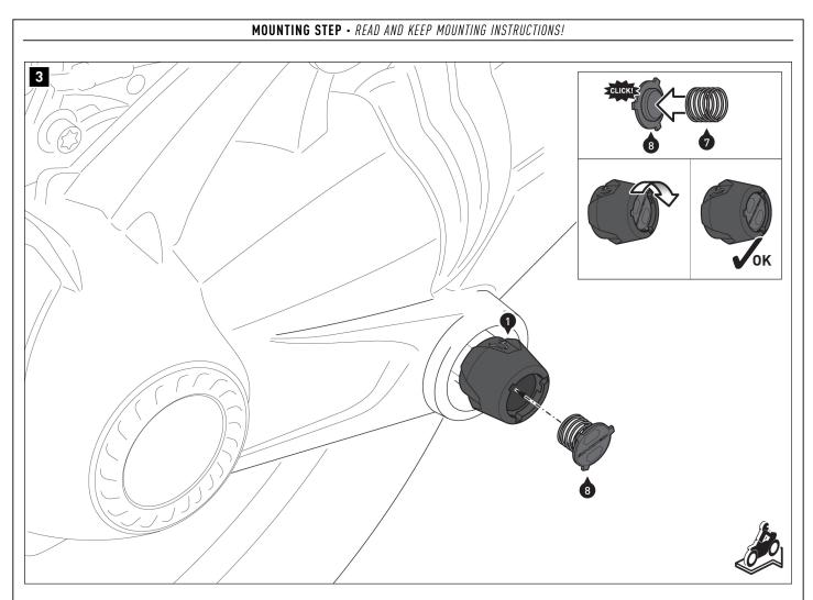
Insert the spring (7) into the cover cap (8) as shown in the detailed drawing.
