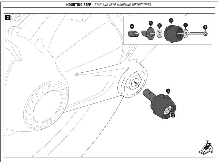
Loosely screw parts (1) to (6) together as shown in the detailed drawing. **A** WARNING: Use low-strength liquid thread locker!
