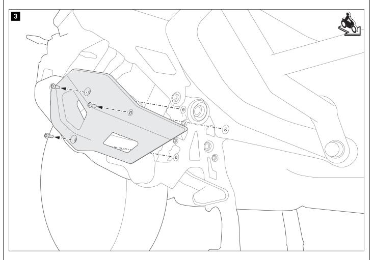
Loosen the screws shown, and remove the heel guard on the right side of the vehicle.
