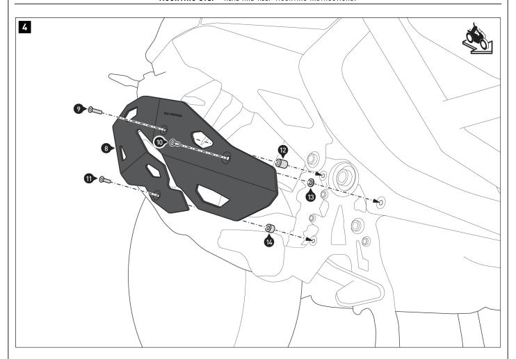
Screw the heel guard onto the right side of the vehicle. **A** WARNING: Use a liquid threadlocker!
