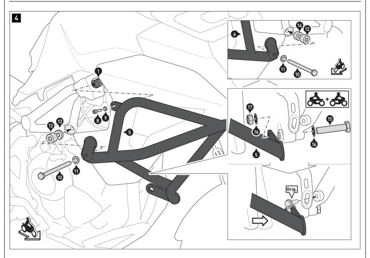
Screw the right-hand crash bar (5) to the vehicle. Note that spacers of different heights are fitted at the rear attachment points on each side.
