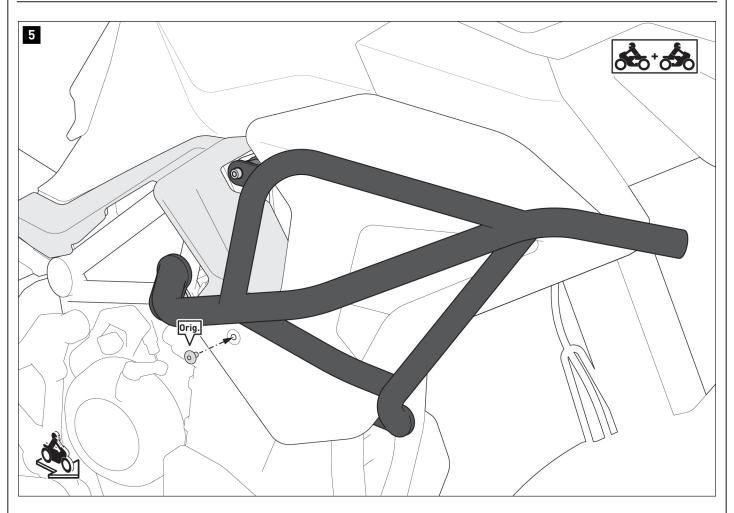
Reattach the side fairings to the vehicle. Tighten the original screw (Orig.) according to the manufacturer's instructions.
