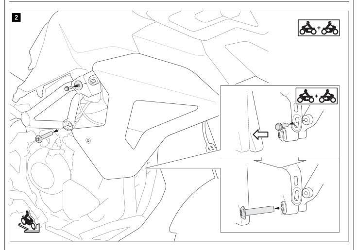
Remove the screws indicated from the vehicle.
