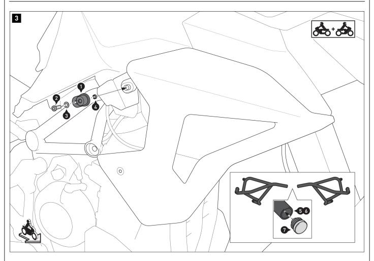
Screw the mounting bracket (1) under the rubber trim to the vehicle. **A WARNING:** Use a liquid threadlocker!
