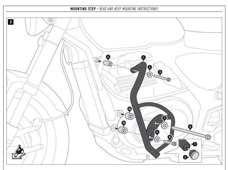
Insert the plastic plug (2) into the openings of the crash bar (1) as shown in the detailed drawing. Screw the **left-hand** crash bar (1) to the vehicle. **A WARNING: Use liquid thread locker (only for screws (3) and (8))!** Tighten screws (3) and (8) according to the vehicle manufacturer's specifications. Do not tighten screw (6) yet.
