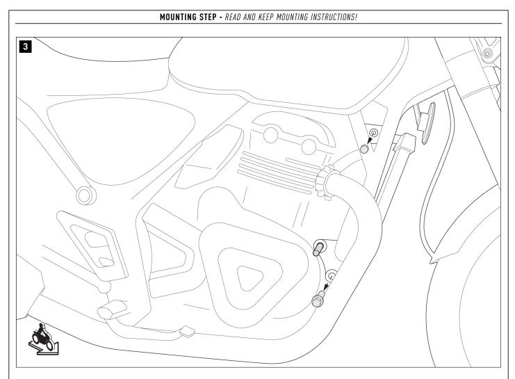
Remove the screw and plastic plug indicated from the vehicle.
