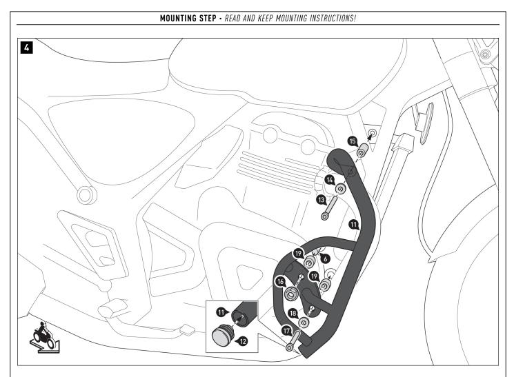
Insert the plastic plug (12) into the openings of the crash bar (11) as shown in the detailed drawing. Screw the **right** crash bar (11) to the vehicle. **A WARNING: Use liquid thread locking agent (only for screws (13) and (17))!**
