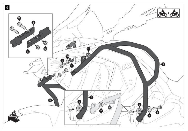
$\triangle$  **NOTE:** If this product is to be installed with the SW-MOTECH crash bar, the installation situation at the lower attachment point changes (see detailed drawing below). Use the screws (\*) included with the crash bar.
