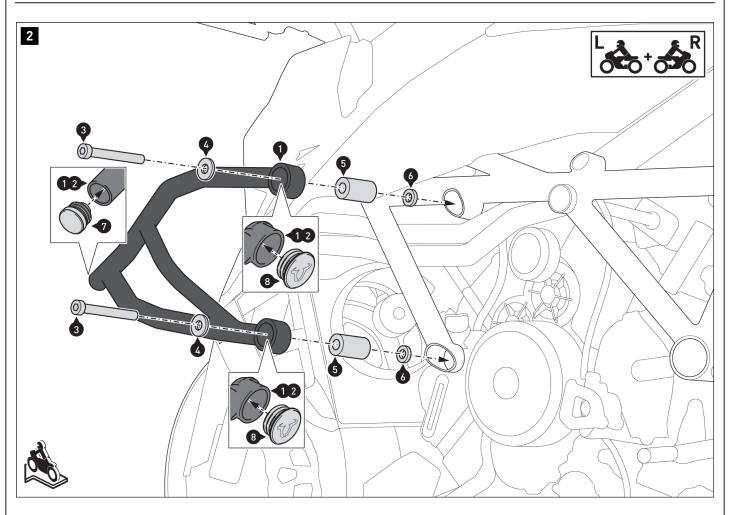
Insert the plastic plugs (7) into the opening of crash bars (1) and (2).
