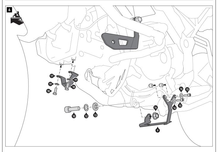
**△NOTE:**Use the screw (11) at the left attachment point when mounting the SW-MOTECH centerstand at the same time. Parts (12) and (13) are omitted. Use the parts on the centerstand instead.
