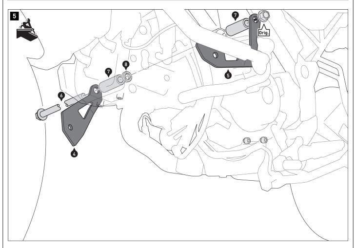
**\_NOTE:**Use the indicated parts when mounting the SW-MOTECH crash bar at the same time. The crash bars are screwed onto the mounting brackets (4) and (5).
