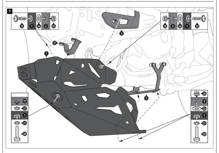
Screw the engine guard (1) to the mounting brackets (4), (5), (9) and (17). **AWARNING:** Use liquid thread locker (front screw (20) only)!
