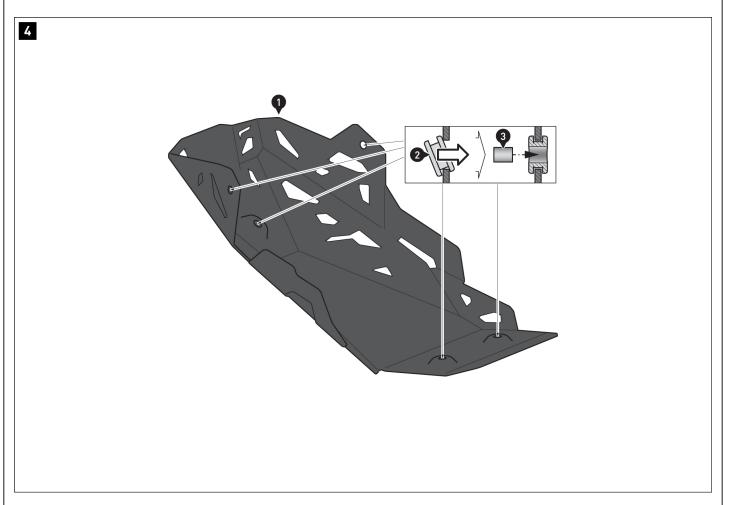
Insert the rubber grommets (2) into the openings of the engine guard (1). Then press the spacers (3) into the openings of the rubber grommets (2).
