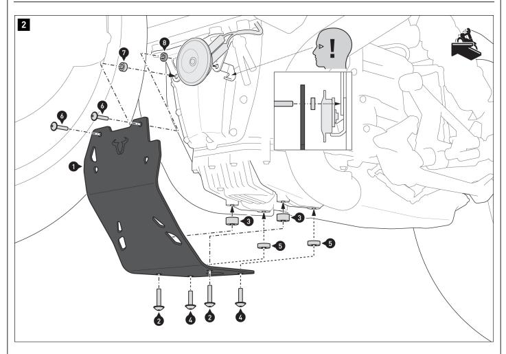
$\triangle$  **NOTE:** Be sure to mount the horn so that it rests on the marked anti-twist lock as it was originally. Otherwise, the horn may become damaged.
