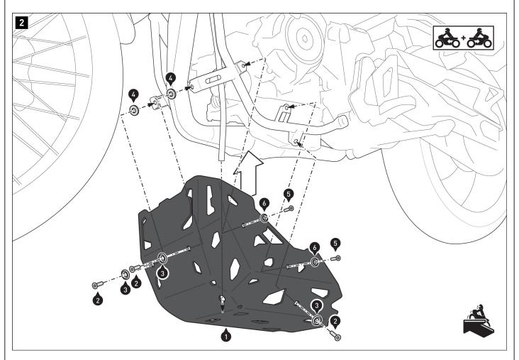
Screw the engine guard (1) to the vehicle.
