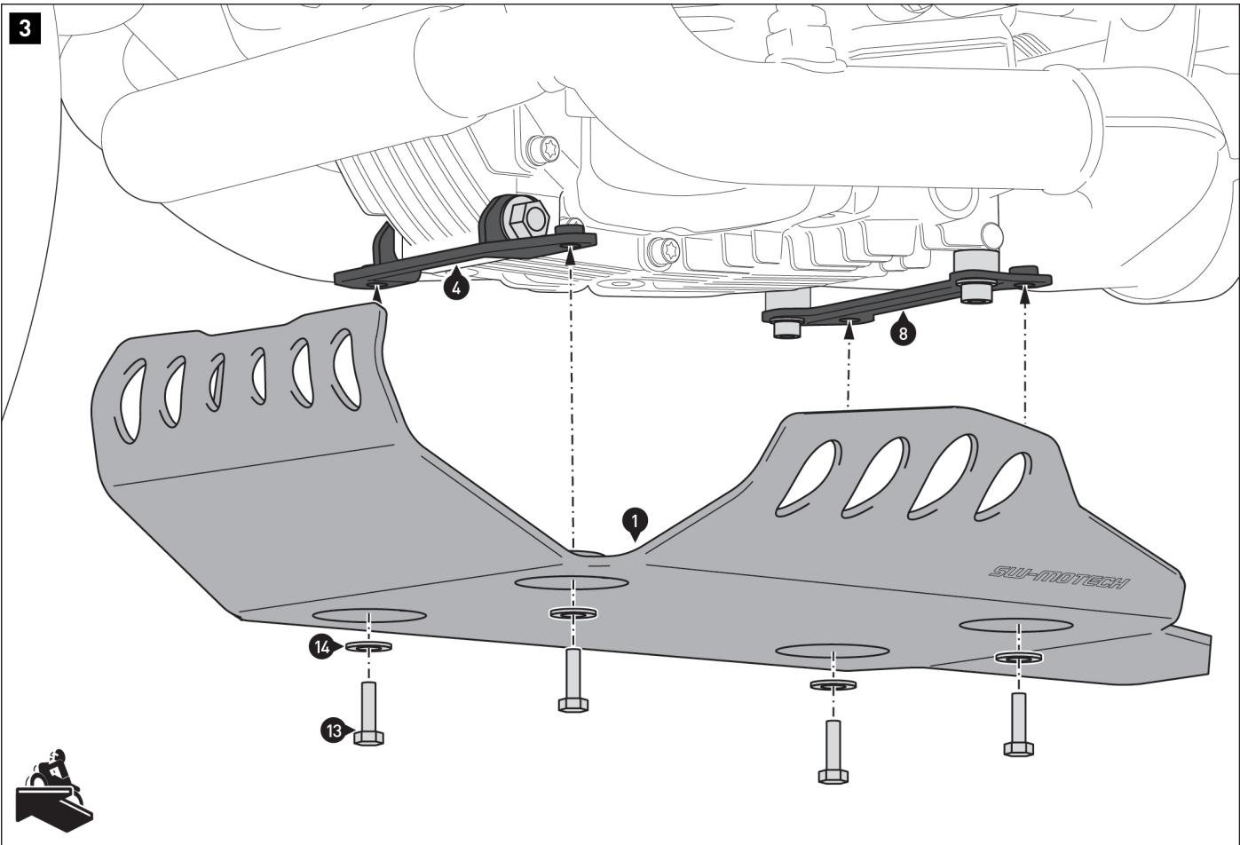
Screw the engine guard (1) to the mounting brackets (4) and (8).
