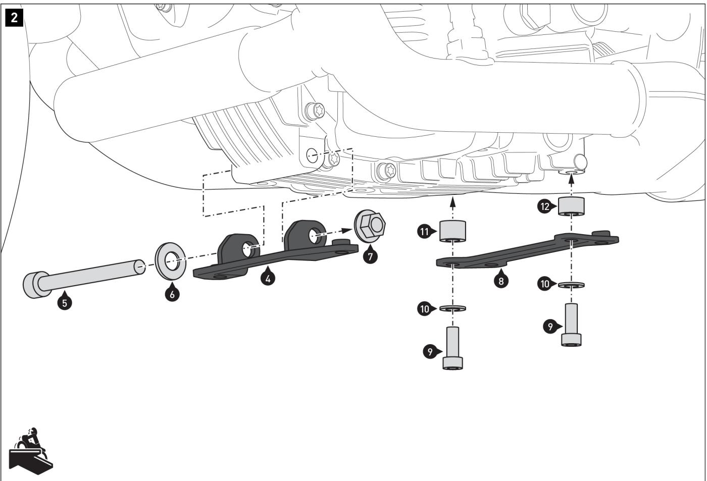
Screw the mounting brackets (4) and (8) to the vehicle.
