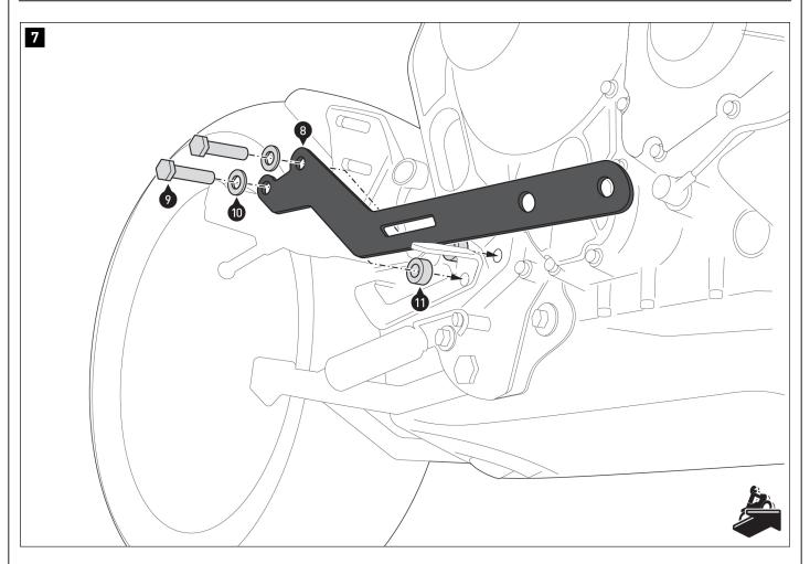
Screw the mounting bracket (8) onto the right side of the vehicle behind the brake lever.
