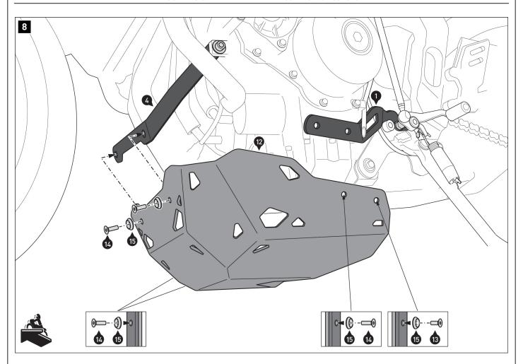
Screw the engine guard (12) onto the mounting brackets (1), (4) and (8). Note the position of the screw (13).
