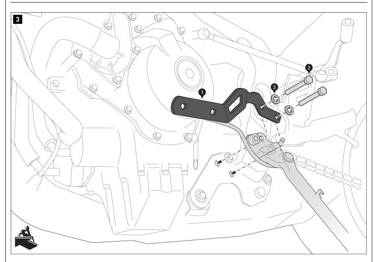
Screw the mounting bracket (1) to the side stand on the left side of the
