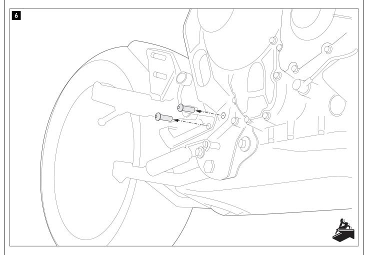
On the right side, remove the two screws as shown in the drawing.
