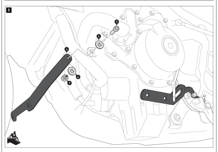
Screw the mounting bracket (4) onto the left side of the vehicle. **A WARNING:** Use liquid threadlocker!
