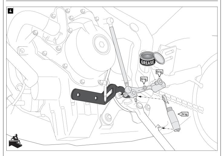
Hook the original tension spring (Orig.) back onto the side stand. Coat the shaft of the original screw (Orig.) with grease. Screw the gear lever back onto the vehicle using the original screw (Orig.). Tighten the original screw (Orig.) according to the manufacturer's instructions.
