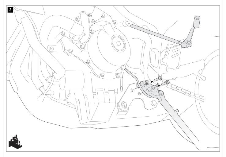
Remove the screw shown and detach the side stand from the mounting bracket.
