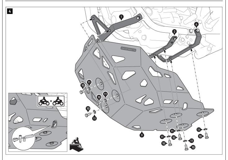
Screw the engine guard [9] to mounting brackets [1], [2] and [6] as shown in the drawing.
