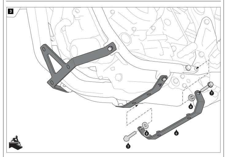
Screw the rear mounting bracket (6) to the vehicle frame. **A WARNING: Use a liquid threadlocker!**Do not tighten the screws (7) yet.
