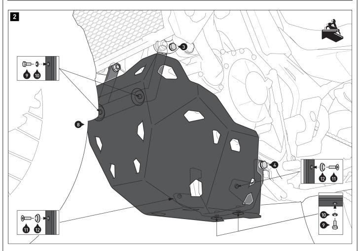
Screw the engine guard [8] to mounting brackets [1] and [2]. **A WARNING:** Use a liquid threadlocker!
