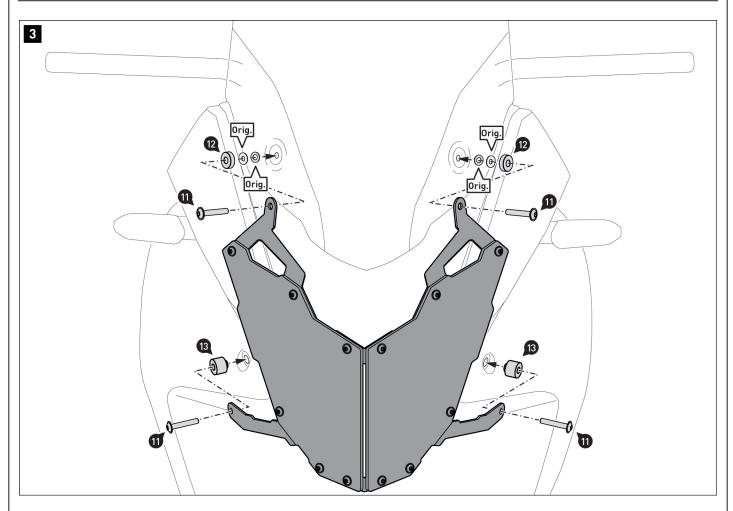
Screw the headlight guard onto the motorcycle. **A NOTE:** Be sure to first mount the rubber washers (Orig.) and then the white PA washers (Orig.).
