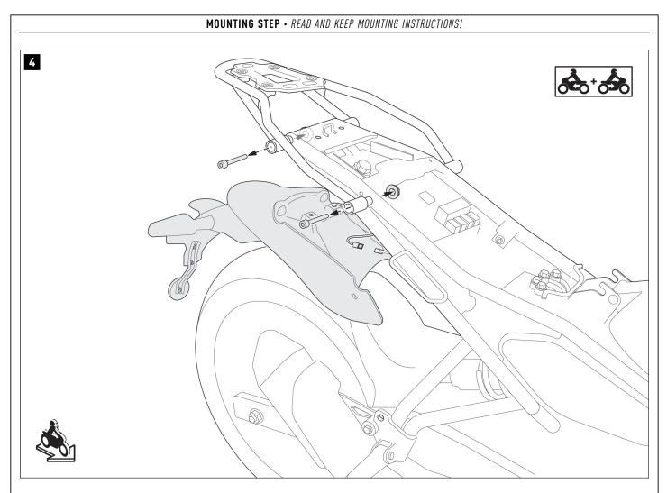
Remove the screws and nuts of the passenger grab handles  $\boldsymbol{\mathsf{on \ both \ sides}}$  .
