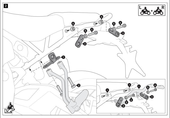
Screw the mounting brackets (1) to the passenger footrests on both sides of
