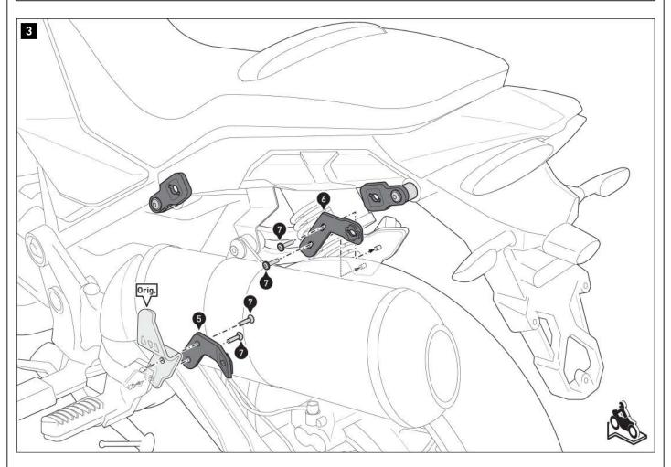
Attach the mounting bracket [5] with the original heat shield (Orig.) ( **left side** of the vehicle ) and the fastening tab [6] (**right side** of the vehicle) on the
