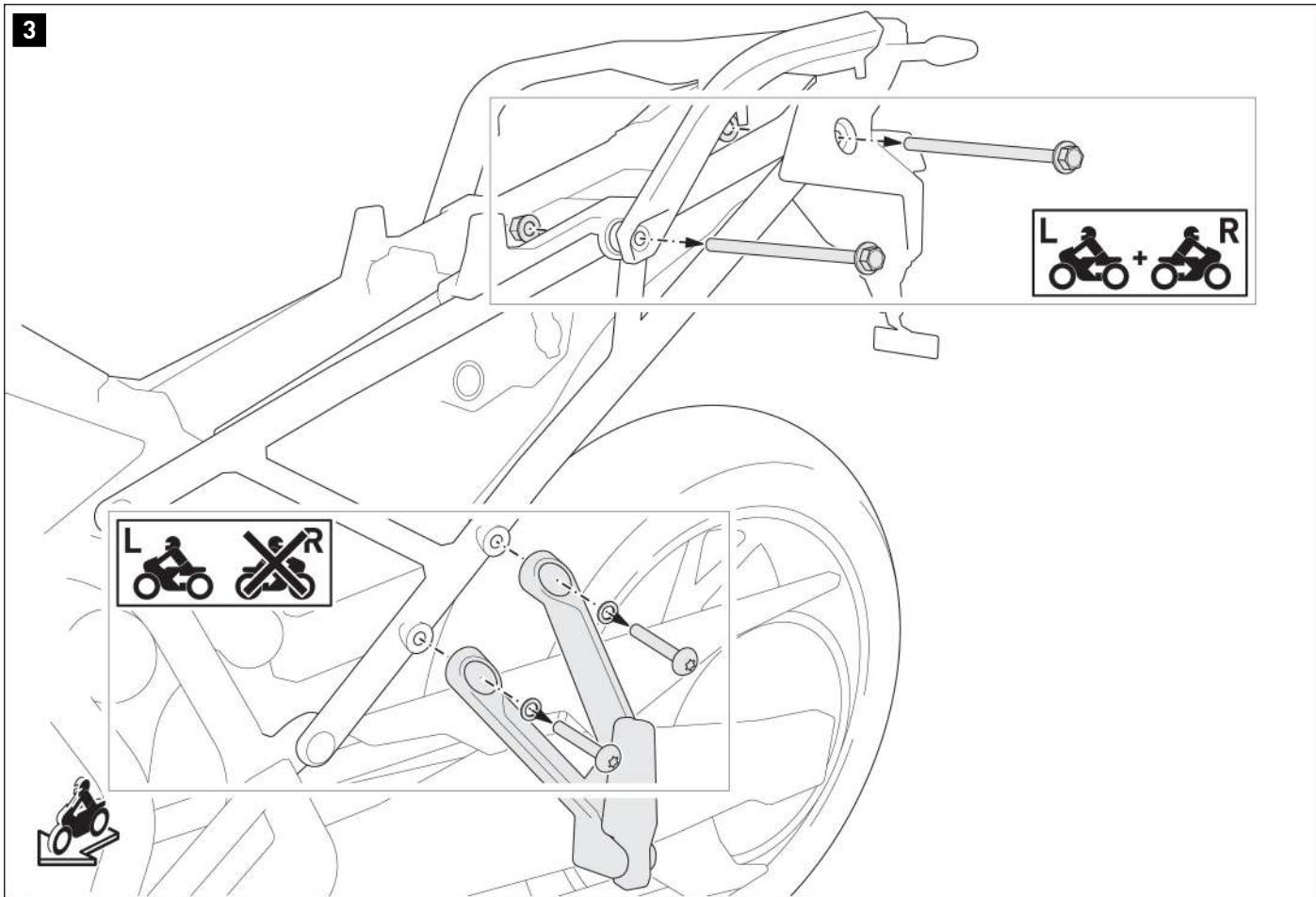
Remove the screws and nuts (as shown in drawing) from both sides of the rear of the vehicle.
