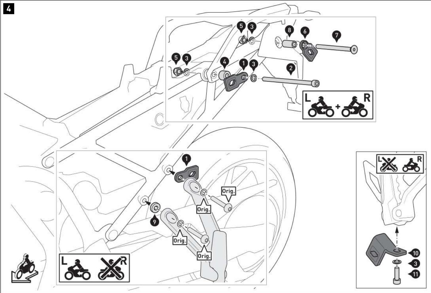
Screw fastening straps (1) and (6) on both sides of the vehicle.
