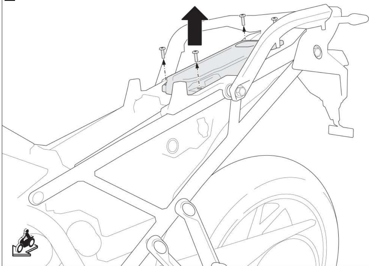
Remove the screws shown, loosen the connector, and remove the control unit with the cover from the vehicle.
