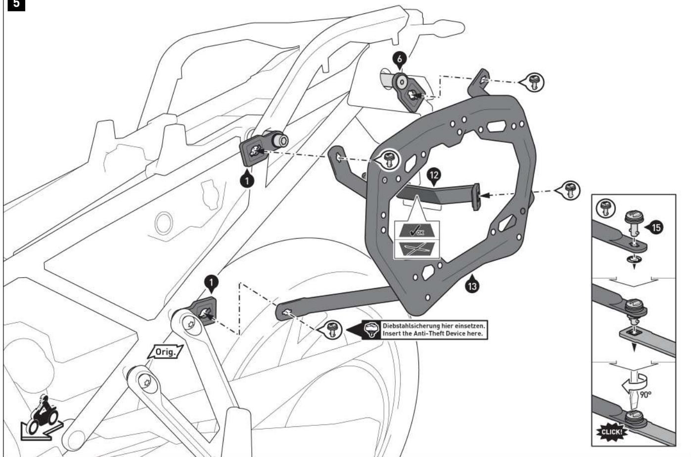
**△ NOTE:** The SW-MOTECH anti-theft protection devices are available separately; mount the anti-theft protection devices on both sides at the marked position.
