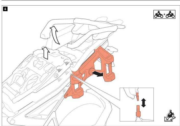
Lift the frame cover and loosen the plugs underneath the original side carriers.
