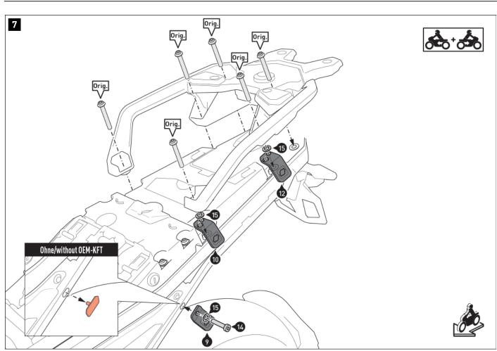
▲ **NOTE:** Pay attention to the hole spacing of the mounting brackets (10/11) and (12/13); the mounting brackets (10/11) with the smaller hole spacing are mounted at the front in the direction of travel, the mounting brackets (12/13) with the larger hole spacing are mounted at the rear in the direction of travel.
