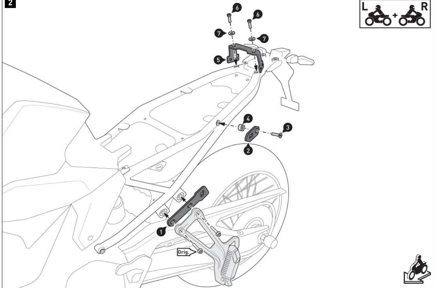
Screw the fastening tabs (1) to the passenger footrests **on both sides**.
