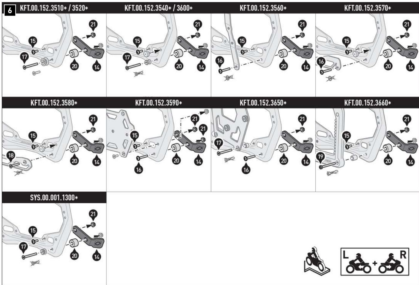
Screw the fastening tabs (14) and the attachment parts for your SW-MOTECH adapter kit to the mounting points shown on the side carriers (11/12). Please follow the mounting instructions for the SW-MOTECH adapter kit.
