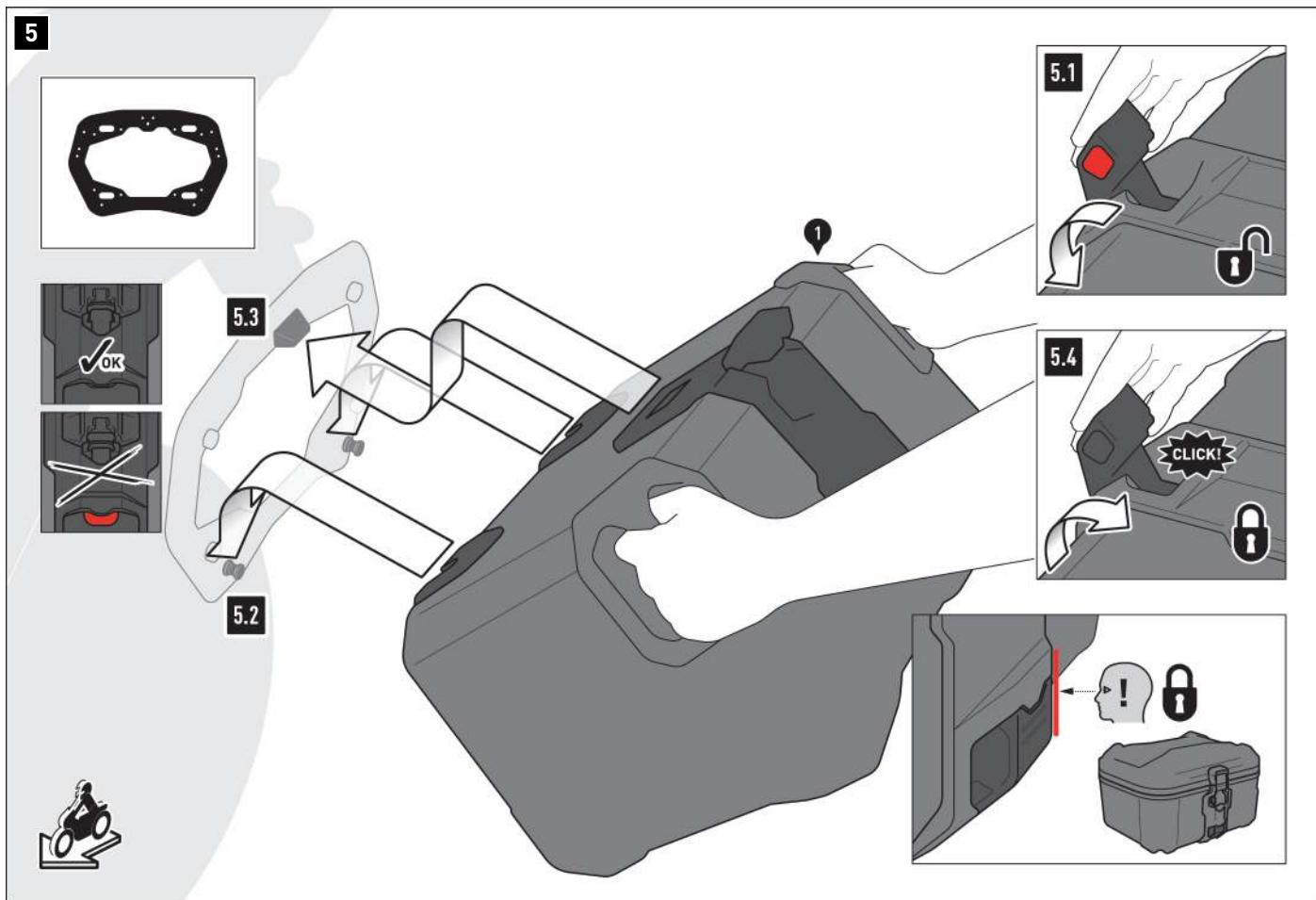
**Attaching the DUSC to a side case**
