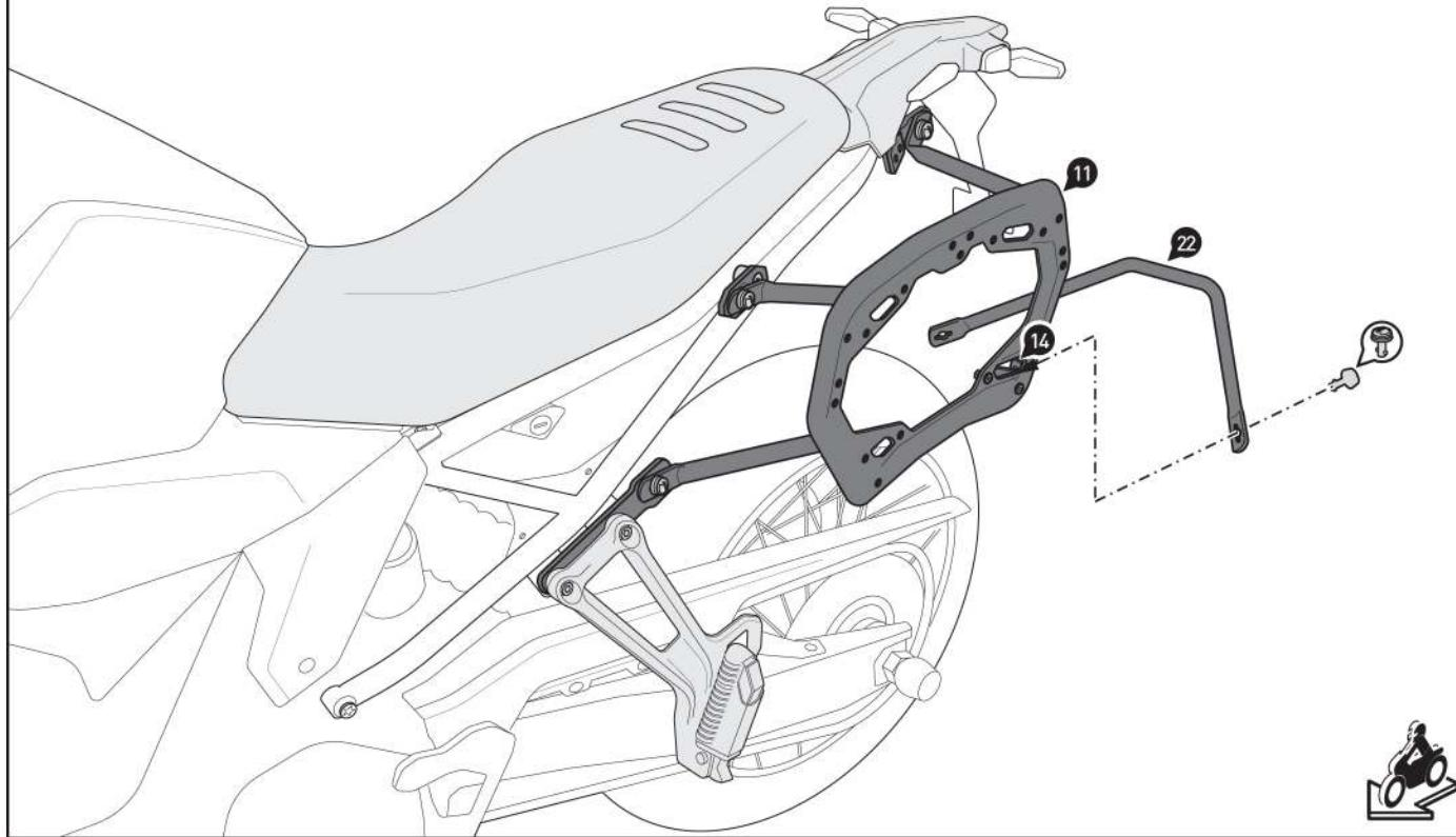
Use the the quick-release fasteners (13) to connect the crossbar (22) **on both sides** to the fastening tabs (14).
