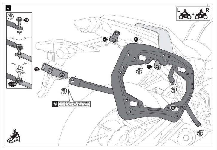
Connect the side carriers (16) and (17) to the mounting brackets (1), (4), (8) and (9) and crossbar (12) using the quick-release fasteners (18). Secure the quick-release fasteners using the lock washers.
