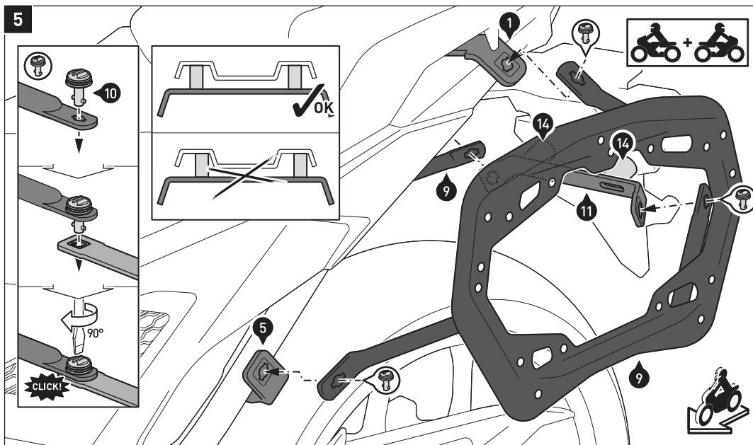
Connect the side carriers (12) to the mounting tabs (2) and (7) by using the fasteners (13), as shown in the detail drawing.
