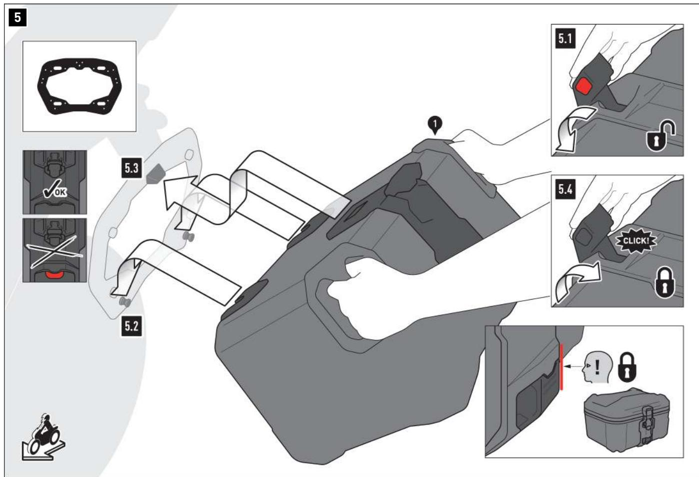
**Attaching the DUSC to a side case**
