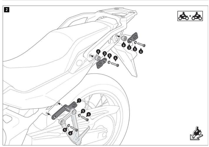
Screw the fastening straps (1), (2) and (3) to both sides of the vehicle. **A WARNING: Use liquid thread locker!** Do not tighten the screws yet.
