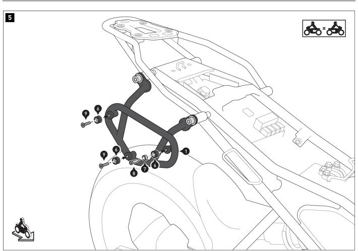
Screw parts (6) to (9) to the side carrier (1). **A** WARNING: Use a liquid threadlocker! Tighten the screws (8) and (9) as specified in the mounting instructions.
