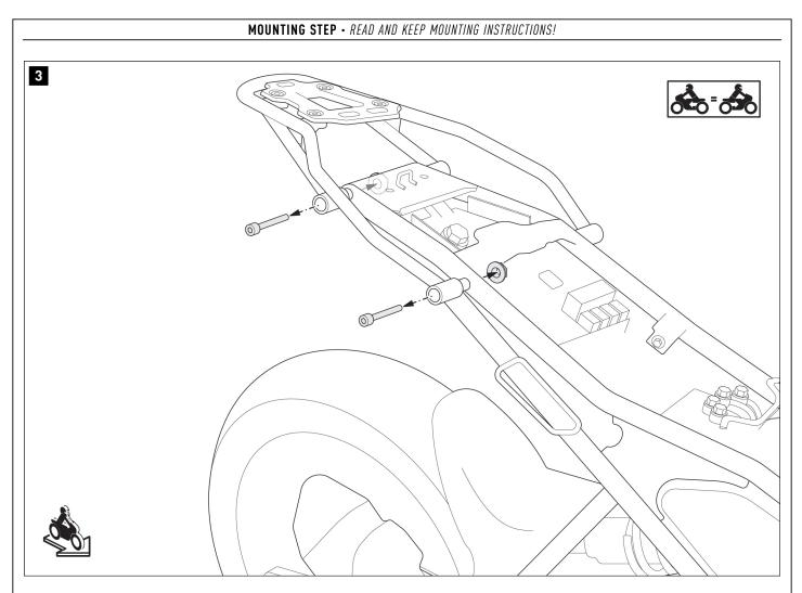
Remove the screws and nuts from both sides of the passenger grab handles.
