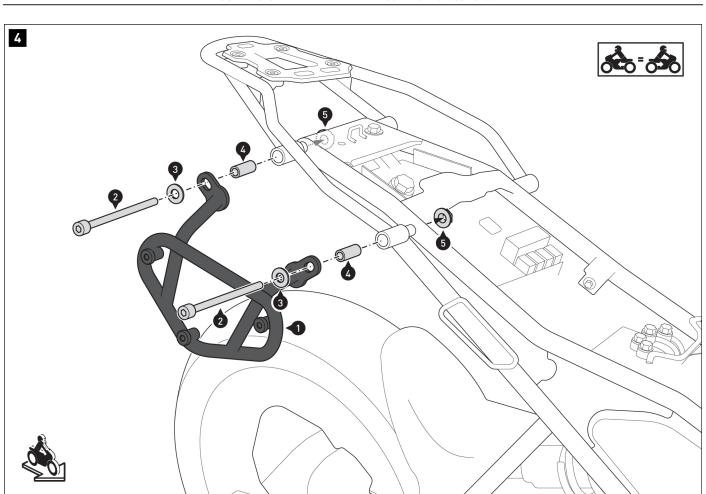
Screw the side carrier (1) to the vehicle using the parts indicated. Tighten the screws (2) as specified in the mounting instructions.
