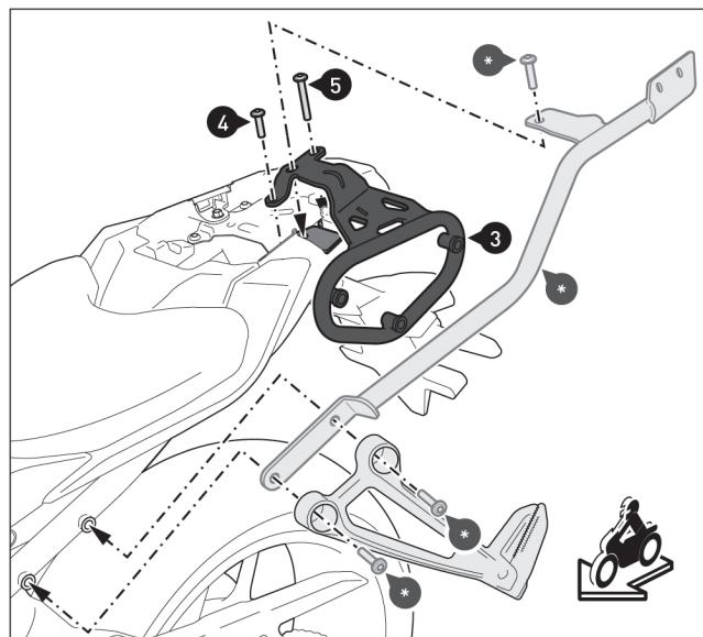
**⚠ NOTE:** The following assembly steps show the assembly of the left side carrier. Install the right side carrier in the same way.
