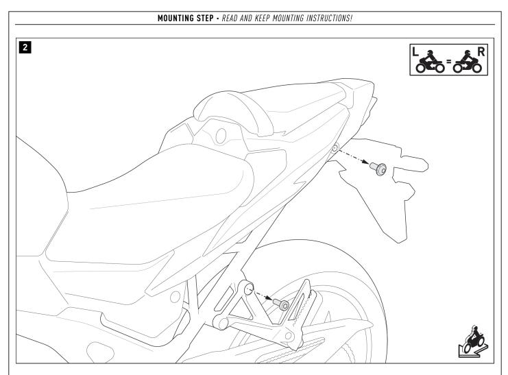
Loosen the screws from the attachment points indicated.
