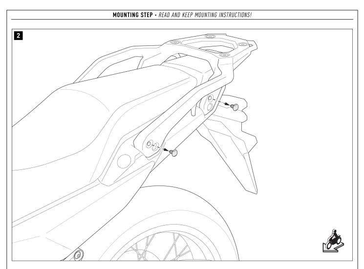
Remove the plastic plugs indicated from the vehicle.
