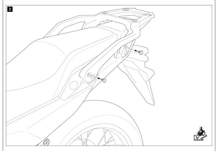
Remove the plastic plugs indicated from the vehicle.
