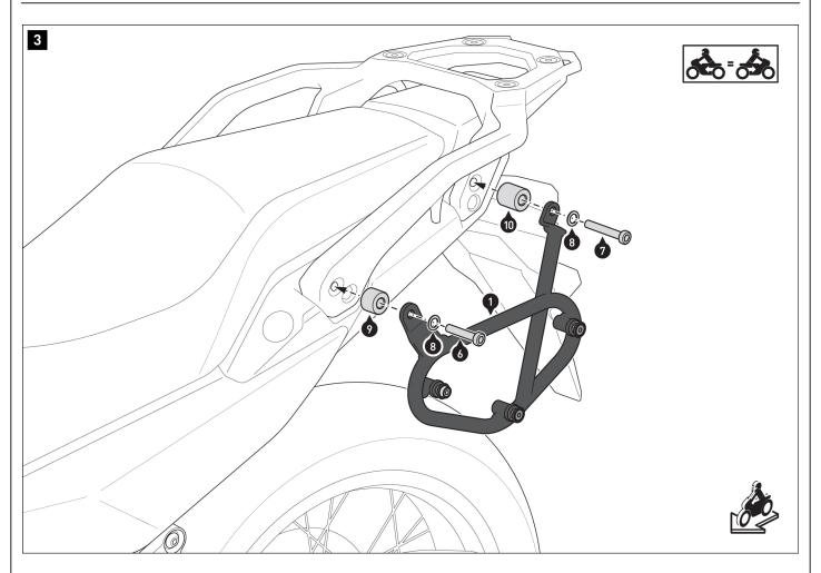
Screw the side carrier (1) to the vehicle.
