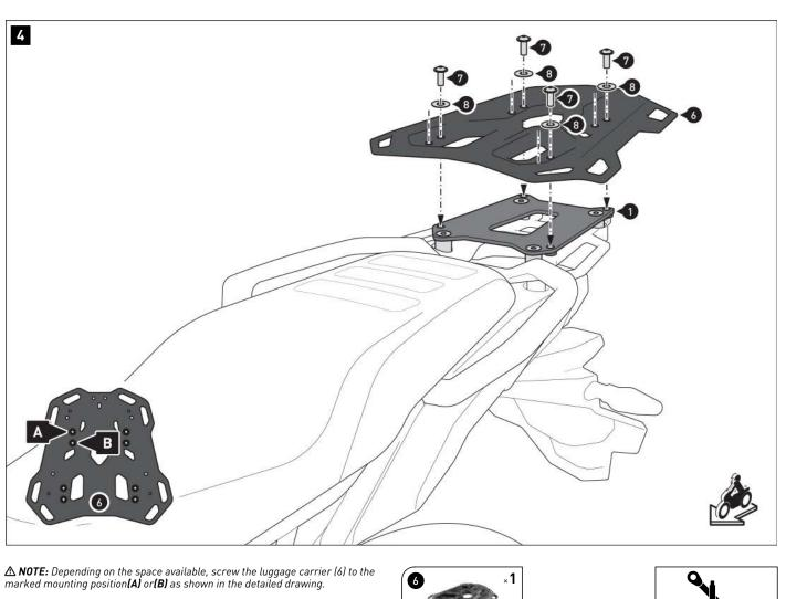
Mount the luggage rack (6) on the mounting plate (1). **A WARNING: Use a liquid threadlocker!** Tighten the screws (7) as specified in the mounting instructions.
