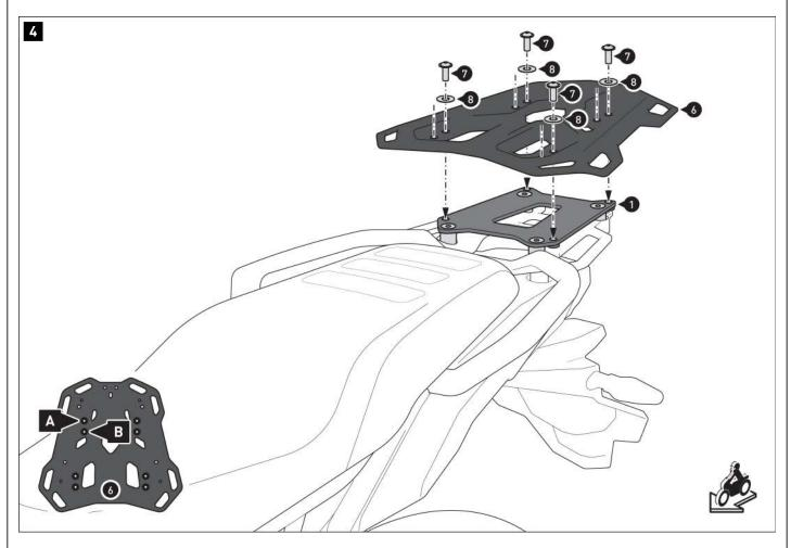
$\triangle$  **NOTE:** Depending on the space available, screw the luggage carrier (6) to the marked mounting position(A) or(B) as shown in the detailed drawing.
