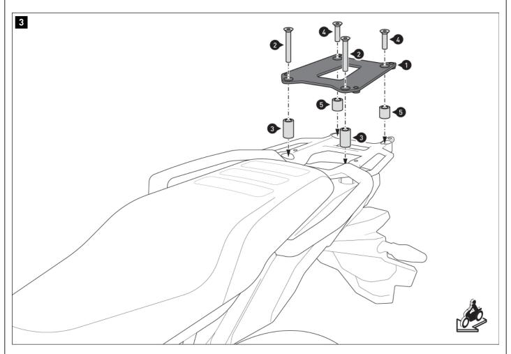
Mount the mounting bracket (1) on the rack.
