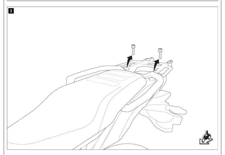
Remove the original screws from the rack.
