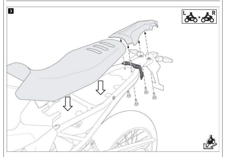
Install the rear cover. Tighten the original screws according to the manufacturer's instructions.
