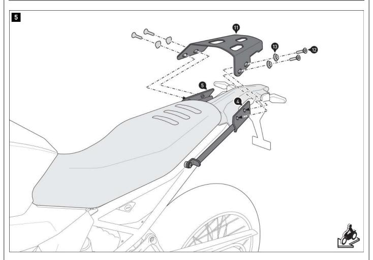
Screw the rack (11) onto the mounting struts [4] and [5]. **A** WARNING: Use liquid threadlocker!
