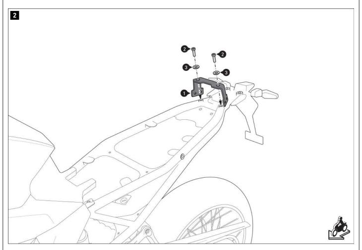
Screw the mounting bracket [1] to the vehicle. **A** WARNING: Use liquid threadlocker!
