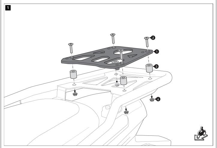
Mount the mounting bracket (1) on the rack. Tighten the screws (2) as specified in the mounting instructions.
