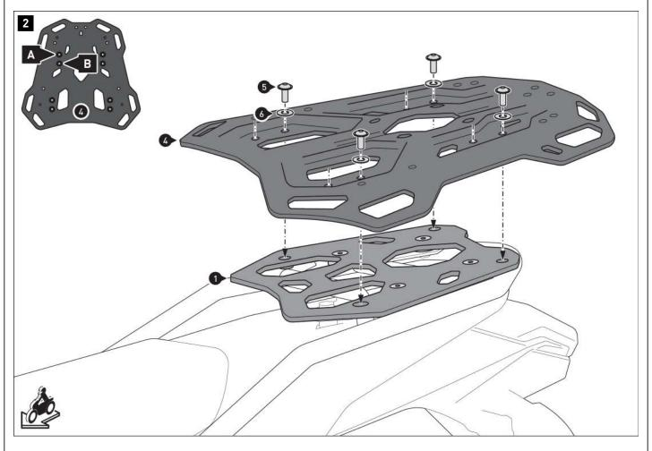
$\triangle$  **NOTE:** Depending on the space available, screw the luggage rack to the marked attachment position (A) or (B) as shown in the detailed drawing.
