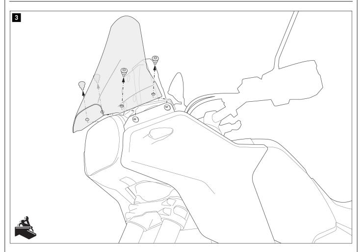
Unscrew the screws shown and remove the windscreen from the vehicle.
