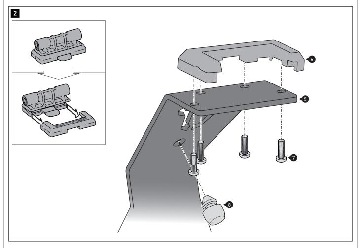
riangle **NOTE:** Holding frame (6) and slide-in frame (2) are delivered assembled!
