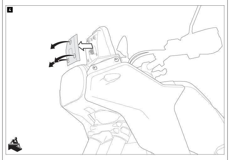
Unscrew the screws and remove the frame cap from the vehicle.
