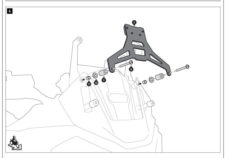
Screw the mounting bracket (5) to the vehicle. **A** WARNING: Use a liquid threadlocker!
