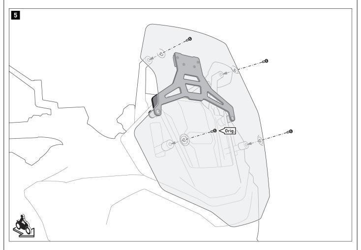
Screw the windscreen back onto the vehicle using the original screws (orig.).
