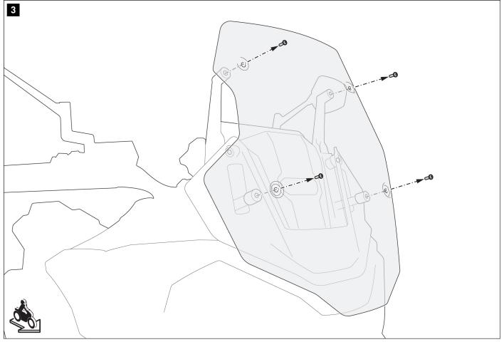
Loosen the screws and remove the windscreen from the vehicle.
