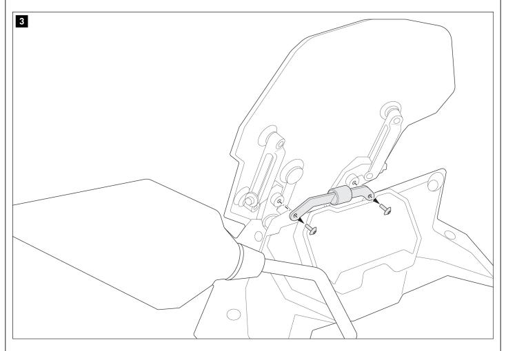
Unscrew the screws shown and remove the component from the vehicle.
