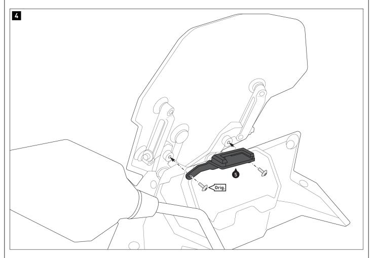
Screw the mounting bracket (5) onto the vehicle using the original (Orig.)
