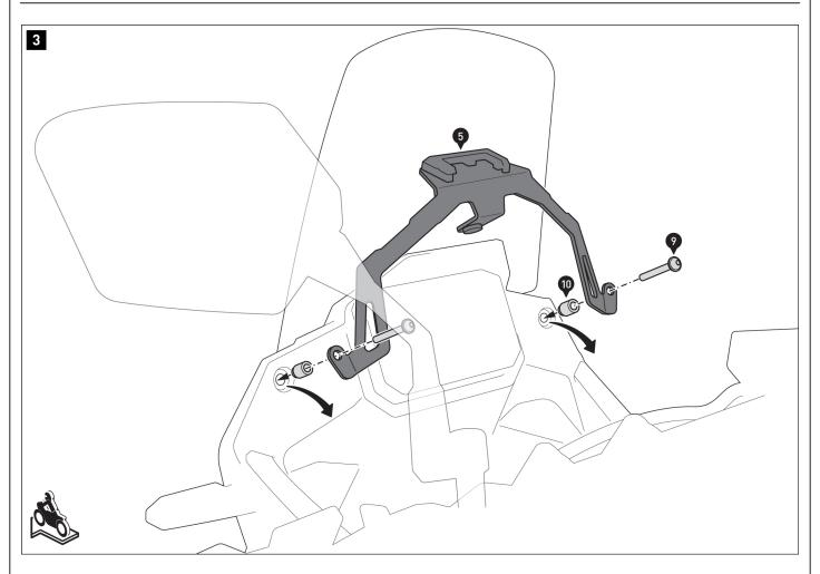
Remove the screws from the attachment points shown.
