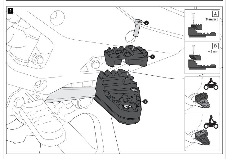
Screw the riser (6) onto the extension (1) in position [A] (standard) or [B] (+ 5
