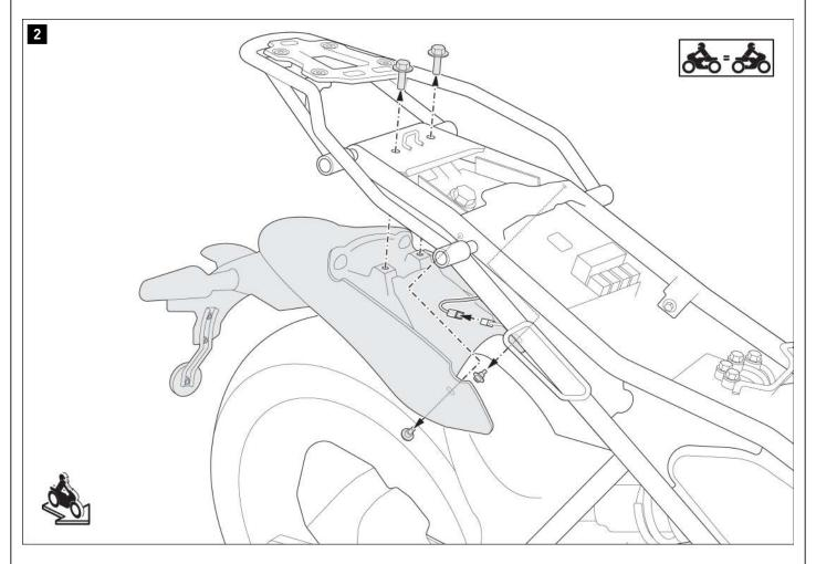
Loosen the four screws on the fender; then disconnect the fender connector.
