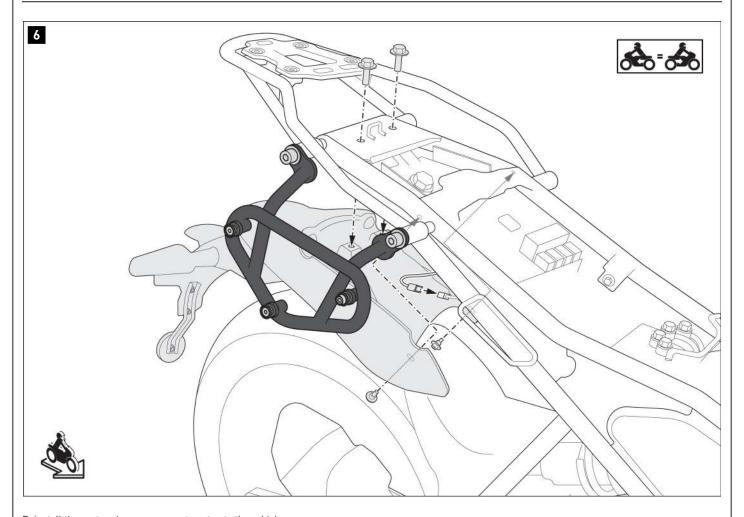
Reinstall the seat and passenger seat seat onto the vehicle. Tighten the original screws according to the vehicle manufacturer's specifications.
