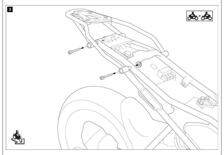
Remove the screws and nuts from both sides of the passenger grab handles.
