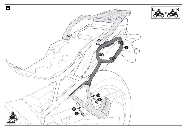
Screw the side support (1) to the footrest on the vehicle. **A WARNING: Use liquid threadlocker!**Now tighten the screws (6) and (9) according to the manufacturer's instructions.
