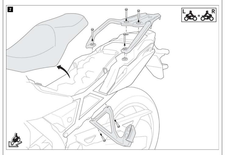
Remove the seat from the vehicle according to the vehicle manual.
