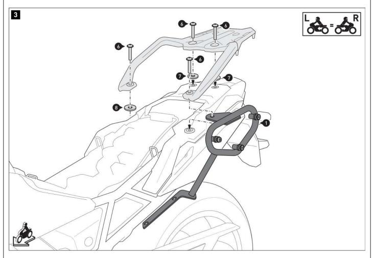
Screw the side carrier (1) to the original luggage rack on the vehicle. **A WARNING:** Use a liquid threadlocker!
