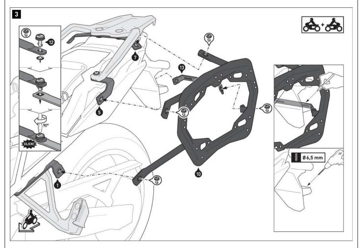
Connect the side carriers (10) and (11) to the fastening straps (1), (2), (5) and (6) and crossbars (7) and (13) using the quick-release fasteners (12). Secure the quick-release fasteners using the lock washers.
