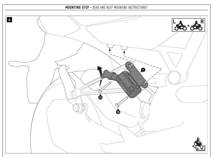
Screw the mounting brackets (1) and (2) to the passenger footpeg bracket on the vehicle. A WARNING: Use a liquid threadlocker! Tighten the original (Orig.) screws according to the manufacturer's instructions.
